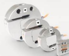
This cost effective S-type laod cell is designed for tank,vessel,hooper weighing and truck scales. It is also used filling,packing and batching applications.Although this load cell is utilized in compression , it is possible to use in tension and also bi-directional forces. Manufactured for weighing 300-10.000 kg capacities. It is possible to use aluminium version of ST load cells for low capacities like 20,50,100 and 200 kg.
