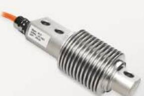
The BT series bending beam is designed for tension or compression loading applications including bench scales,conveyor weighing and gravimetric filling machines.The stainless steel bellow construction makes the complete system impervious to hostile environments and washdown applications.Manufactured for weighing 10-500 kg capacities.
