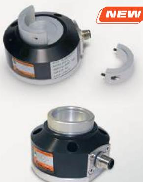
RS Series load cell is designed for measuring the tension in winding drum applications. It senses the applied force to the bearing of loadcell which is mounted at the edge of the drum during the process of winding and unwinding. It is widely used in textile and printing industry. Manufactured for weighing 25,50 and 100 kg capacities.
