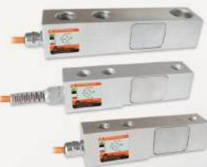
This single ended shear beam load cell is designed for high capacity automatic fillingmachines.It can be used in weighing platforms by the change of up side down. Manufactured for Weighing 300-5.000 kg capacities.
